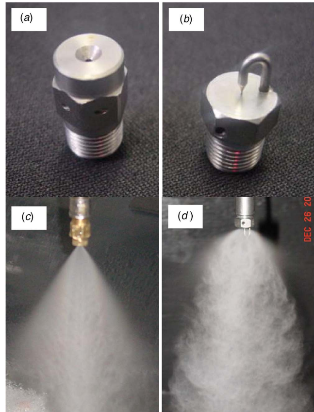
Fig. 5 (a) Swirl nozzle (b) impaction pin nozzle; plume characteristics at operating pressure of 138 barg (2000 psig): (c) swirl jet nozzle and (d) impaction pin nozzle [16]
