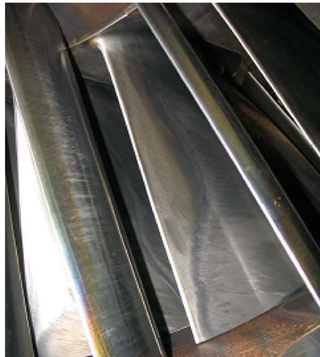
Fig. 8 Blade condition of first stage compressor blades of AL-STOM advanced heavy duty industrial gas turbine GT24 (Courtesy Caldwell Energy & Environmental, Inc.)
