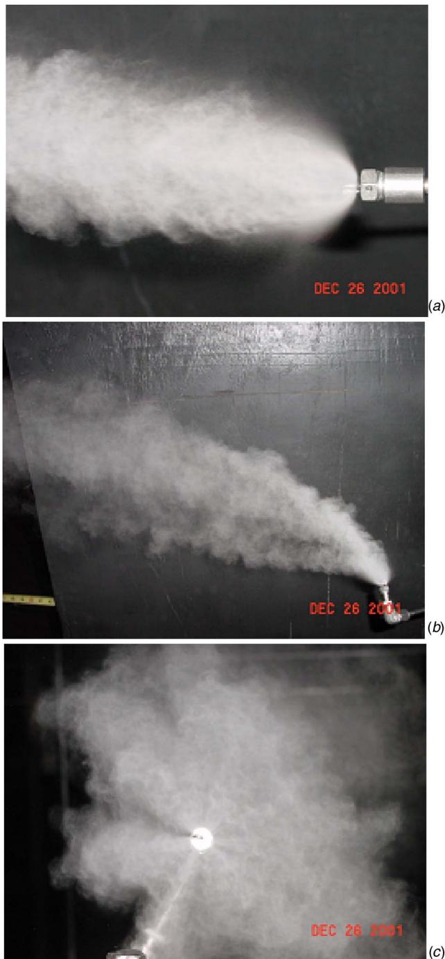
Fig. 17 (a), (b), and (c) Plume shape with nozzle orientation of a fog nozzle in the wind tunnel; airflow velocity is 4 m/s (800 ft/min), Operating pressure is 138 barg (2000 psig): (a) Co-flow; (b) 90 deg; (c) counter-flow
